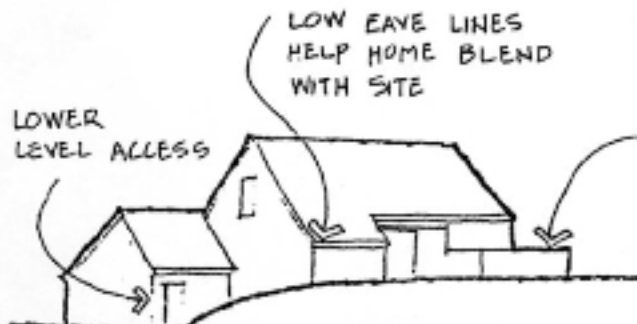
Gable Roof on Hillside
